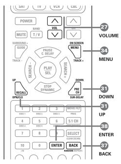
The following buttons are used to navigate the ON-SCREEN MENU system:
